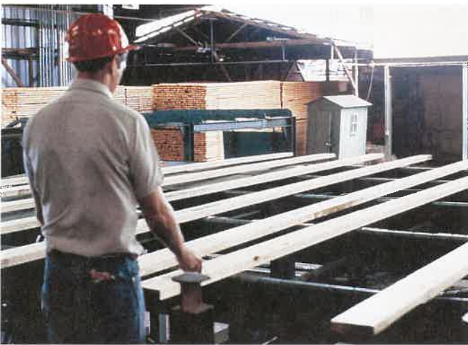
Figure 11-22. Graders inspect each board for size and clearness. (Southern Forest Products Assoc.)
