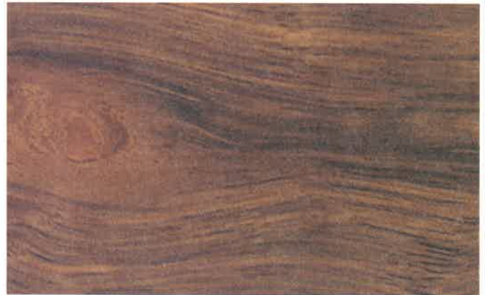
Figure 12-26. Paldao is comparable to walnut in appearance and working qualities. It is considered an exotic wood and used primarily for architectural woodwork.
