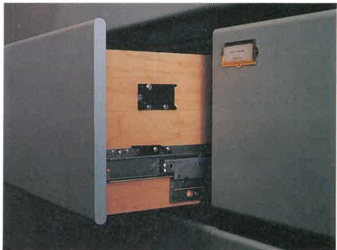
Figure 14-18. Postforming of radius edges and matching PVC edging eliminates the dark brown line. The top and bottom edges of the drawer front serve as the drawer pulls. (Chuck Davis Cabinets)
