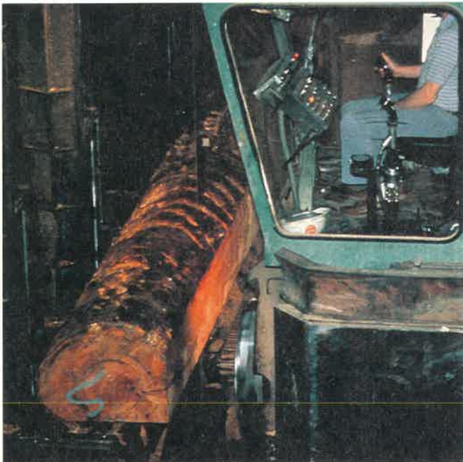
Figure 11-5. Logs are mounted on a carriage to be sawn. The carriage is moving the log along a band saw. (Western Wood Products Assoc.)
