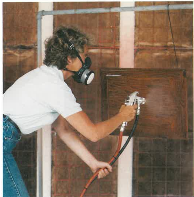
Figure 6-15. Spraying is an efficient method of applying finishing materials. (ITW DeVilbiss)
