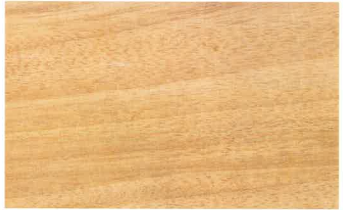
Figure 12-31. Primavera resembles mahogany in grain pattern. However, it is much lighter in color.
