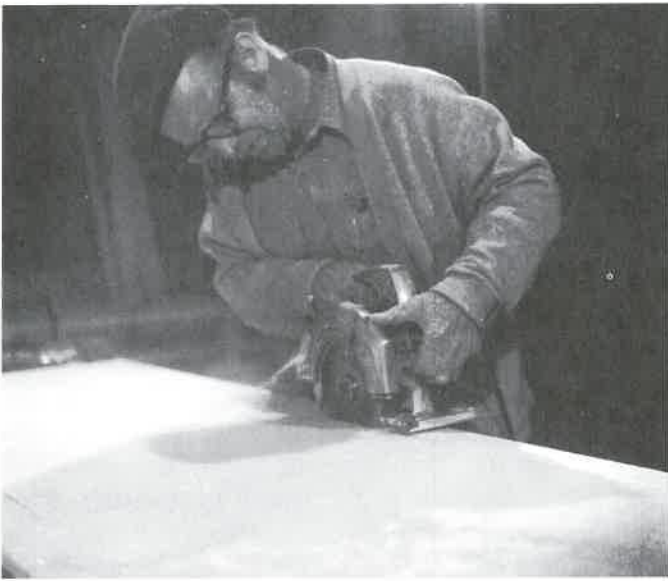
Figure 15-35. Plastic tops are cut and shaped with conventional woodworking tools. Use carbide tipped saw blades and router bits. (DuPont)
