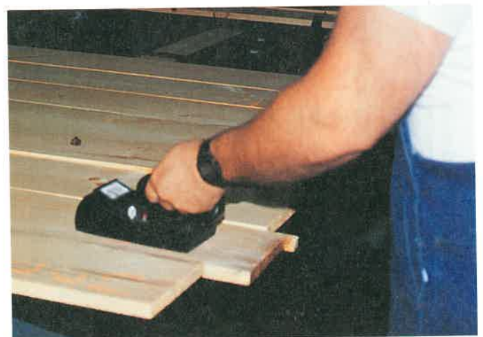
Figure 10-9. Moisture content of wood can be determined by a moisture meter. Insert probes in the wood to obtain a reading. (Western Wood Products Assoc.)
