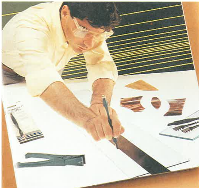
Figure 15-5. Glass is scored with a glass cutter. A straight edge serves as a guide for scoring straight lines. (The Fletcher-Terry Co.)
