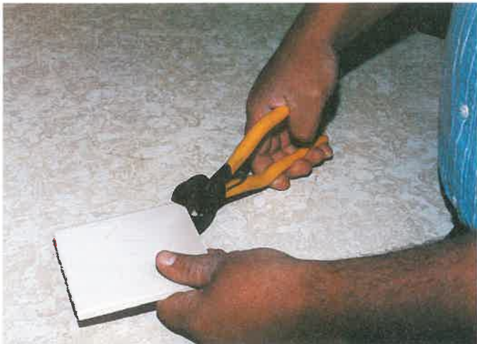
Figure 15-40. Tile nippers chip off bits of tile for irregular shapes.
