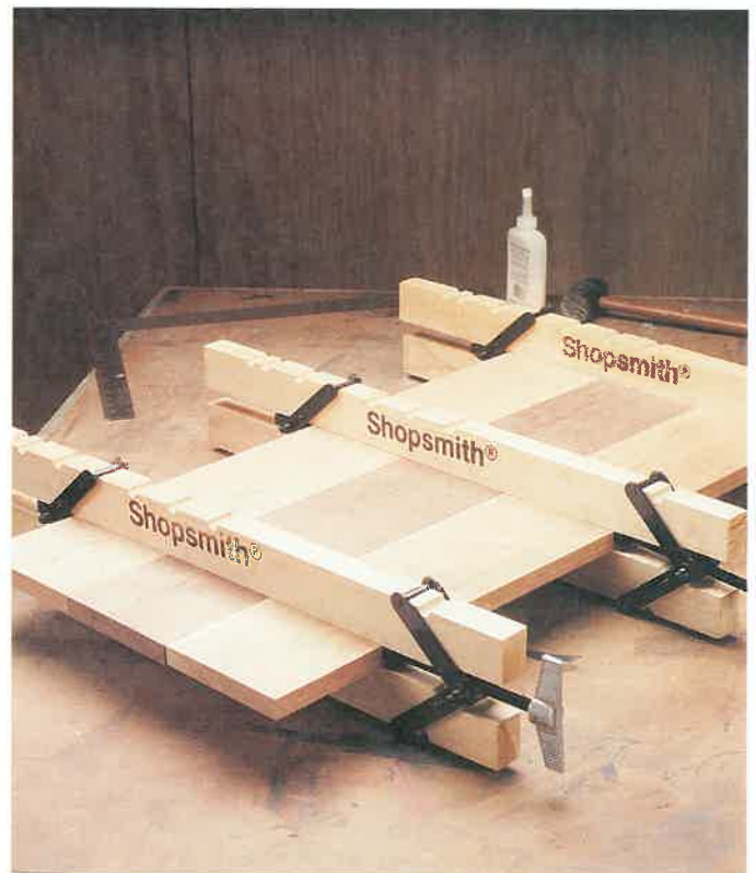
Figure 6-14. These double bar clamps consist of two radiused hardwood bars and are fully adjustable to varying lengths of stock. They provide clamping on a full range of widths and simultaneously apply pressure from sides, top, and bottom when pieces are glued edge-to-edge. (Shopsmith)
