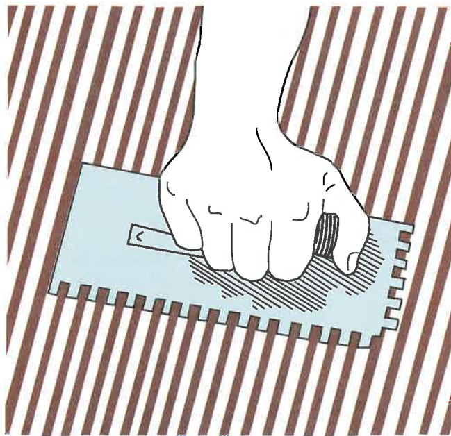
Figure 15-38. A notched trowel spreads mastic evenly.
