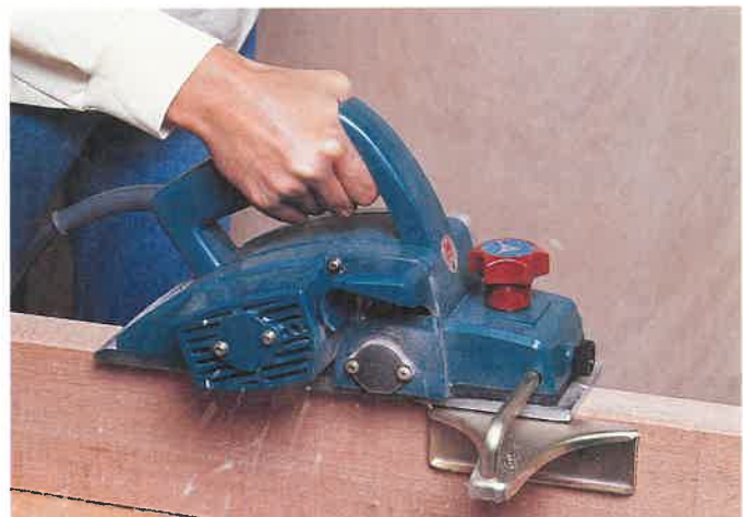
Figure 6-8. A portable power planer works well for narrow faces and edges. (Makita U.S.A., Inc.)
