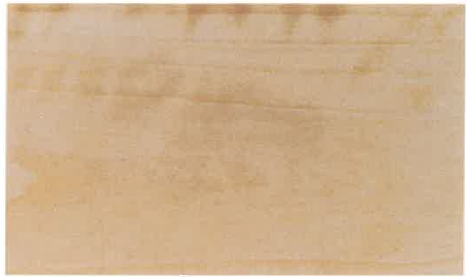
Figure 12-11. Cottonwood is soft and light in weight, but difficult to split. (Fine Hardwood Veneer Assoc.)
