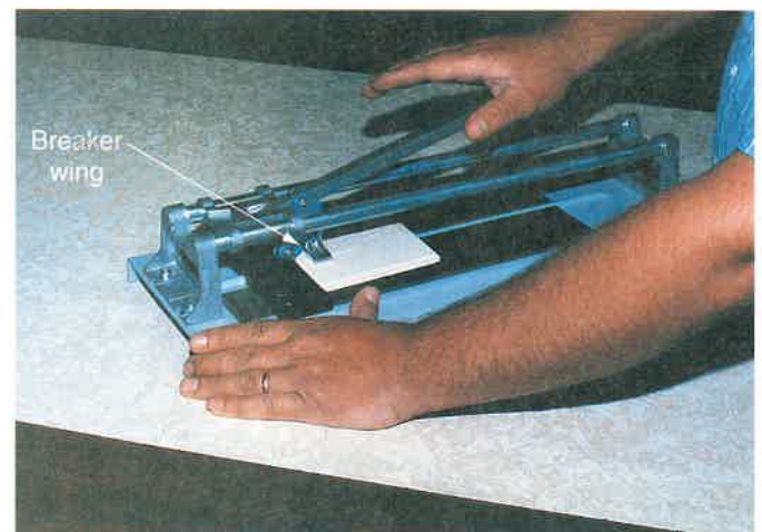
Figure 15-39. A tile cutter scores and breaks tile easily. A—Place marked tile in cutter. Pull the handle toward you to score the tile. B—Locate the breaker wing over the tile and push the handle down to fracture the workpiece.
