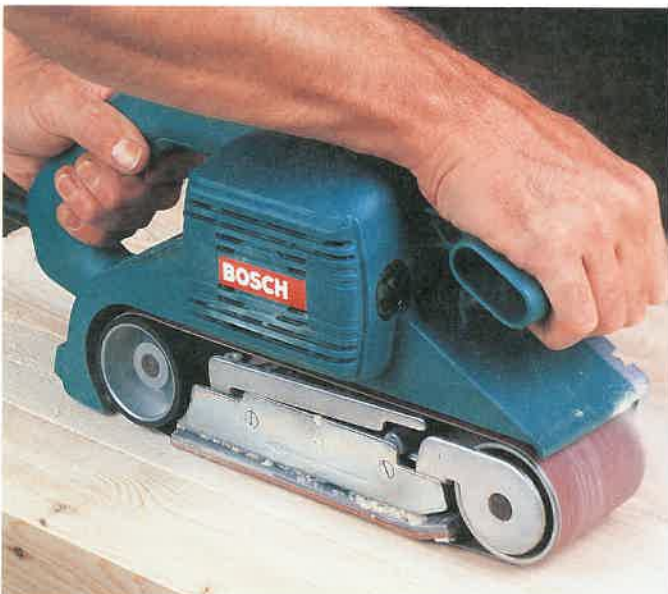
Figure 6-13. Smoothing a surface with a portable belt sander. (Robert Bosch Power Tool Corp.)
