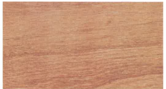
Figure 12-9. Cherry is one of the most popular hardwoods. It sands exceptionally smooth and has a high luster. ( Fine Hardwood Veneer Assoc. )
