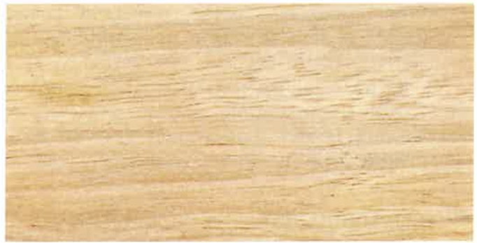
Figure 12-20. Limba, because of its blonde color, is often selected for contemporary furniture.
