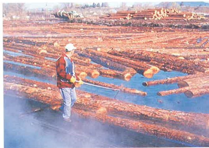
Figure 11-3. Water may be used for transporting and storing logs. (Western Wood Products Assoc.)
