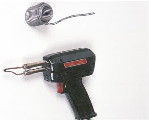
Figure 15-19. A soldering gun or iron melts the solder to bond the lead came.
