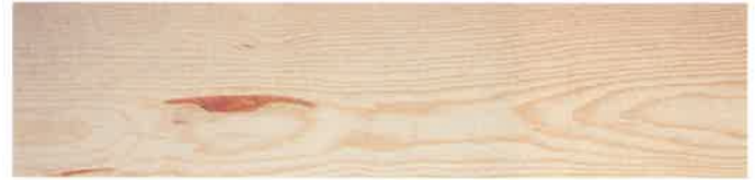
Figure 11-11. Pitch pockets include hardened resins. (Western Wood Products Assoc.)
