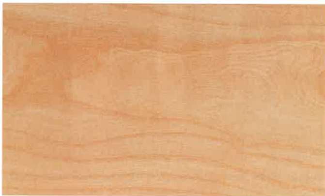
Figure 12-17. Hackberry, a member of the elm family, is often substituted for American elm. ( Fine Hardwood Veneer Assoc. )
