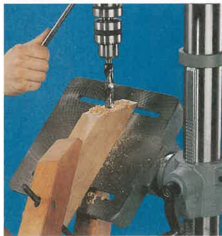
Figure 1-13. Typical processes in cabinetmaking. A—Resawing. ( Delta International Machinery Corp. ) B—Drilling. C—Sanding. ( Delta International Machinery Corp. )
