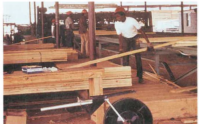
Figure 11-25. Boards are sorted according to grade. (Southern Forest Products Assoc.)
