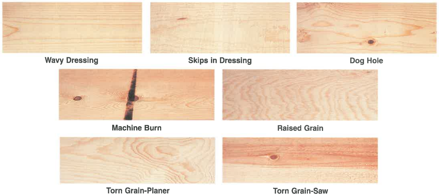
Figure 11-21. Various machine-caused defects occur during surfacing. (Western Wood Products Assoc.)
