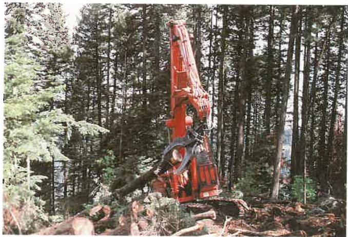
Figure 11-1. After felling, a log loader is used to stack the lumber. ( Western Wood Products Assoc. )
