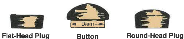
Figure 11-36. Plugs and buttons cover counter bored holes.
