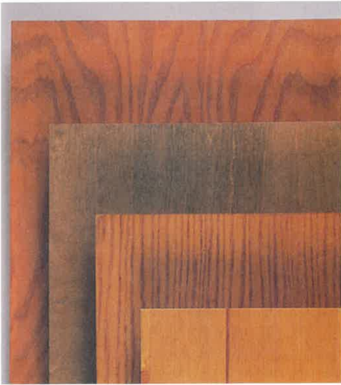
Figure 13-14. Hardwood plywood is fabricated with hardwood face veneers for use where appearance is important. (Georgia-Pacific Corp.)
