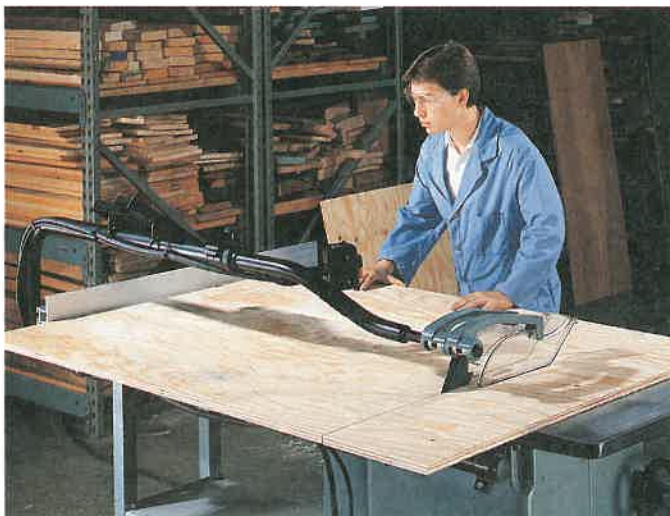
Figure 1-9. Reducing sheets of plywood to component sizes with a table saw. ( Delta International Machinery Corp. )
