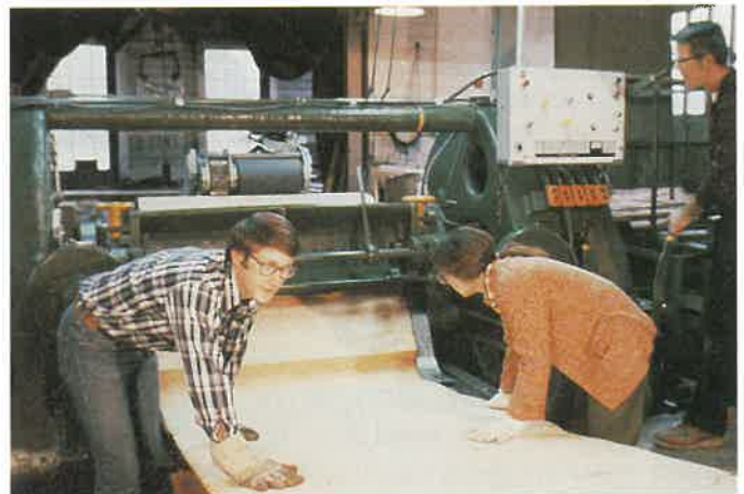
Figure 14-5. Backup rollers turn the log as they press it against the knife. Continuous cutting action produces long sheets of veneer.
