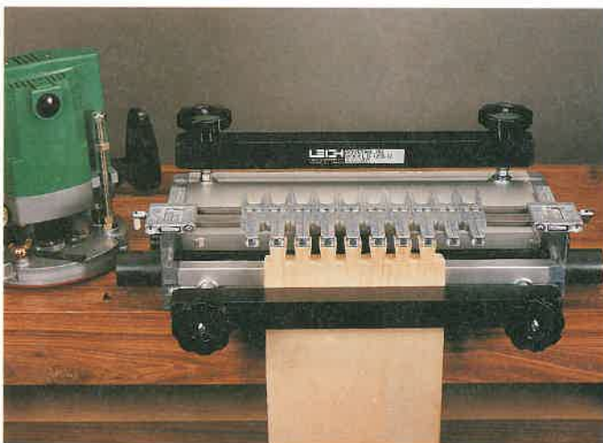
Figure 6-5. A dovetail jig both holds the workpiece and guides the router to make a dovetail joint. ( The Fine Tool Shops )
