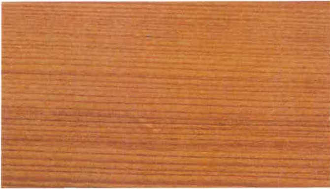
Figure 12-32. Redwood is very resistant to decay. It is widely used for siding and outdoor furniture.
