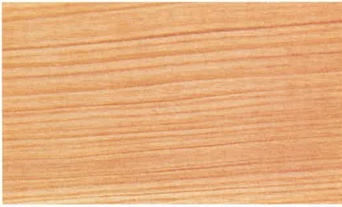
Figure 12-12. Cypress is very durable when placed in a decay-promoting environment.
