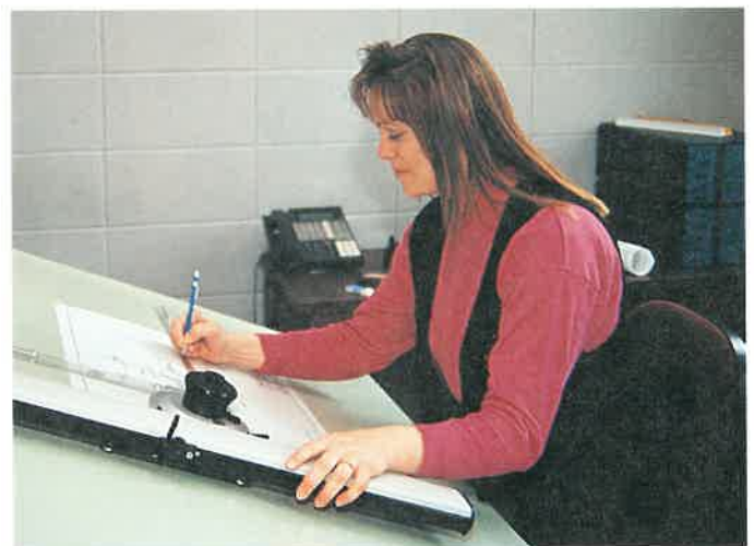
Figure 9-6. Drafting machines combine the functions of a T-square, triangle, and scale. This machine is mounted to a table that may be tilted to a comfortable angle.
