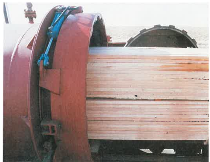
Figure 11-28. Wood preservatives are applied in a high pressure container. (Georgia-Pacific Corp.)
