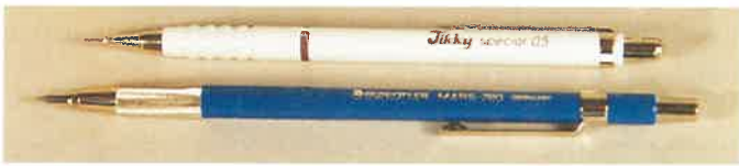
Figure 9-7. Lead holders. Top—Thin leads maintain a fine line. Bottom—Thick leads must be sharpened
