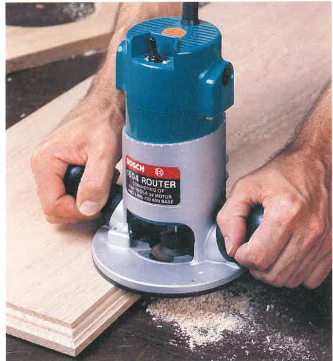
Figure 6-12. Edge designs are created with a portable router and bit. (Robert Bosch Power Tool Corp.)
