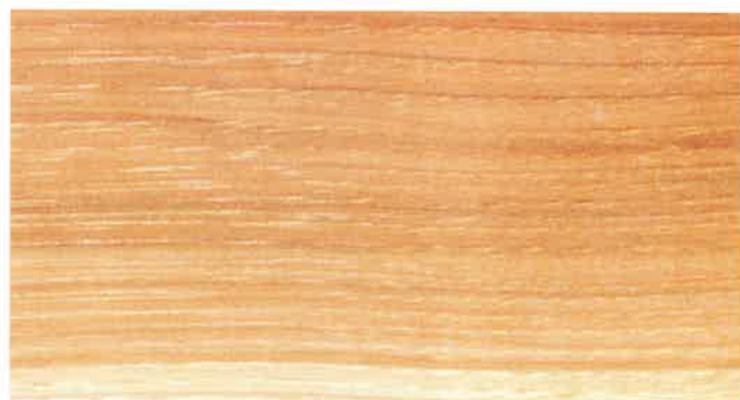
Figure 12-18. Hickory is strong and elastic. It is valued for bent laminations, such as skis. ( Fine Hardwood Veneer Assoc. )
