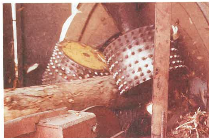
Figure 11-4. Bark is removed before sawing. It will be used to make other products. (Southern Forest Products Assoc.)
