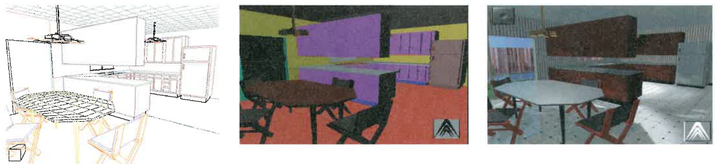
Figure 9-3. Left—The drawing made to look as if it were real. Middle—Color and shading can be added to give more definition to the drawing. Right—Added lighting, textures, and colors give a photographic-quality representation of the drawing. (Autodesk, Inc.)
