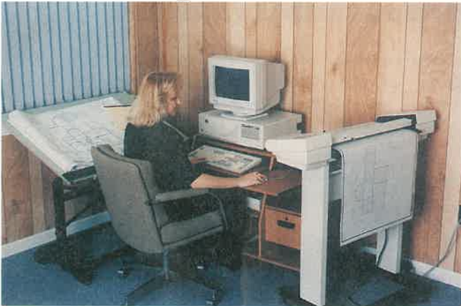
Figure 1-6. Computer-aided design systems help cabinet designers determine size and layout of cabinetry. ( Alpine Structures )
