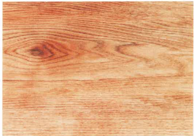
Figure 12-7. Butternut has a light brown heartwood. It is easy to work and machines well. ( Fine Hardwood Veneer Assoc. )
