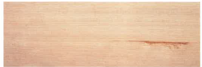
Figure 11-12. Bark pockets are formed when bark cells are enclosed during growth. (Western Wood Products Assoc.)
