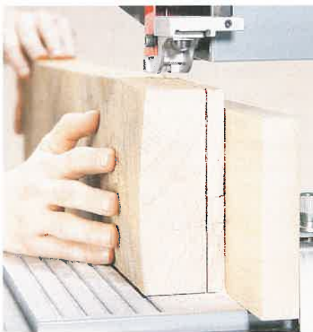
Figure 1-13. Typical processes in cabinetmaking. A—Resawing. ( Delta International Machinery Corp. ) B—Drilling. C—Sanding. ( Delta International Machinery Corp. )
