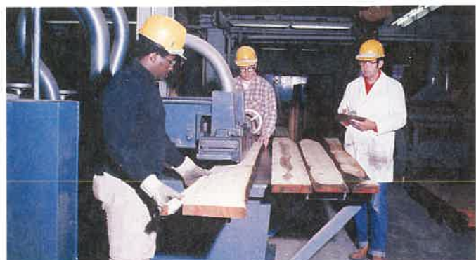
Figure 11-7. Flitches are ripped manually to maximize width. (Forest Products Laboratory)
